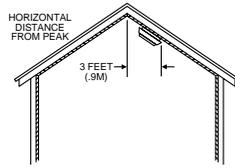
**Where Smoke-alarms Should NOT Be Installed**
